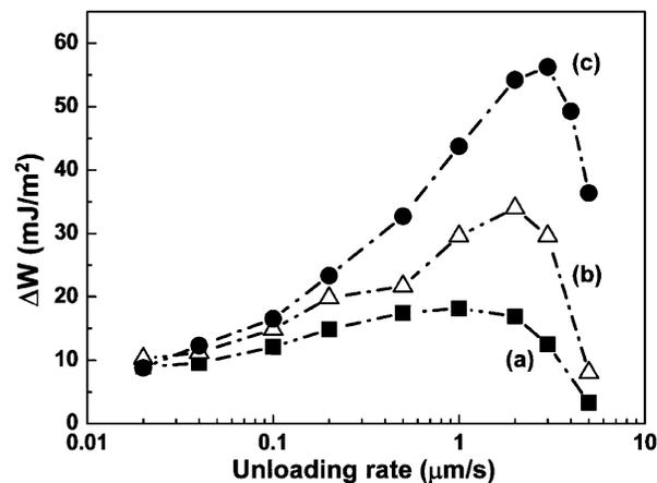
**Figure 4.** Rate dependence on adhesion hysteresis of C-18 monolayers deposited at (a) 5 °C, (b) 30 °C, and (c) 50 °C, respectively. As the monolayer phase approaches a disordered state, the adhesion hysteresis increases, with maximum hysteresis occurring at higher unloading rates.
