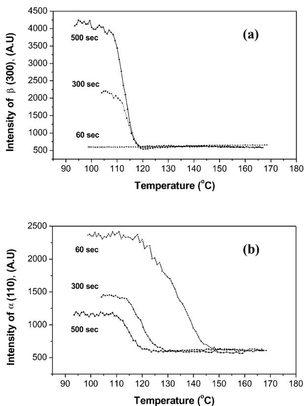
Fig. 9. XRD peak intensities of the  $\beta(300)$  plane and  $\alpha(110)$  plane peaks as a function of temperature for samples prepared at a hold temperature of  $T_h = 168^\circ\text{C}$  and a range of hold times ( $t_h$ ); (a)  $\beta$ -form and (b)  $\alpha$ -form.
