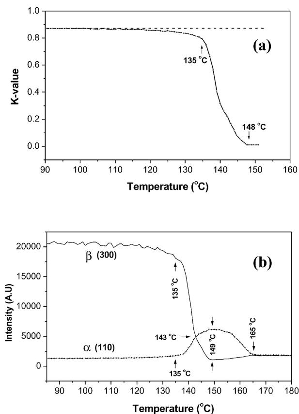
Fig. 5. (a)  $K$ -value as a function of temperature during the melting of  $\beta$ -iPP. (b) XRD peak intensities of the  $\beta(300)$  and  $\alpha(110)$  plane peaks as a function of temperature during the melting procedure.
