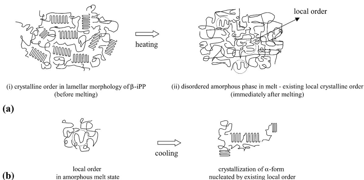
Fig. 3. (a) Schematic representation of crystalline order in  $\beta$ -iPP; (i) before melting, (ii) local order immediately after melting (b)  $\alpha$ -nucleation initiated by existing local order in the melt during the cooling process.
