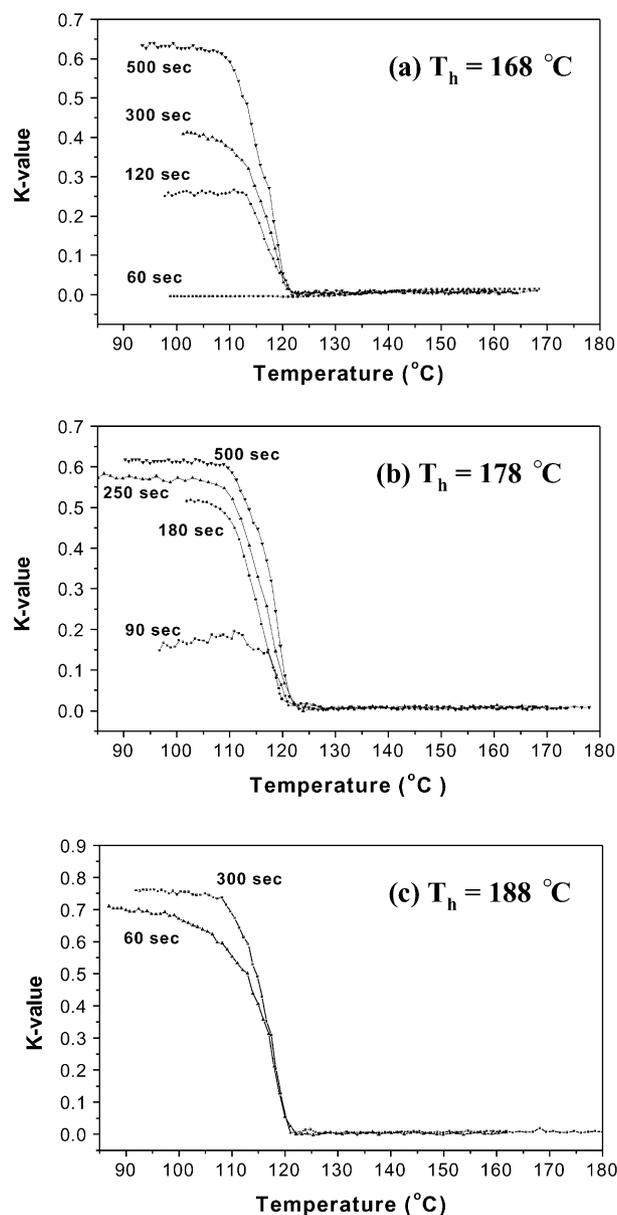
Fig. 8. K-value as a function of temperature during crystallization from samples prepared at hold temperatures (a)  $T_h = 168$  °C, (b)  $T_h = 178$  °C and (c)  $T_h = 188$  °C for different hold times ( $t_h$ ).
