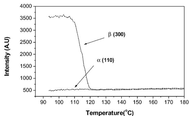
Fig. 6. XRD peak intensities of the  $\beta(300)$  and  $\alpha(110)$  plane peaks as a function of temperature during the crystallization procedure from the sample prepared at  $T_h = 188$  °C,  $t_h = 60$  s.
