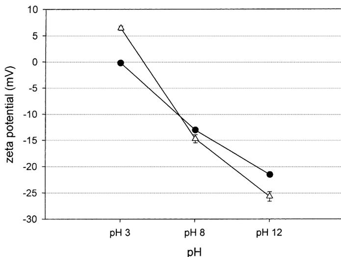
Fig. 5. Zeta potential of untreated polysulfone membrane (●) and oxygen plasma treated polysulfone membrane (Δ).
