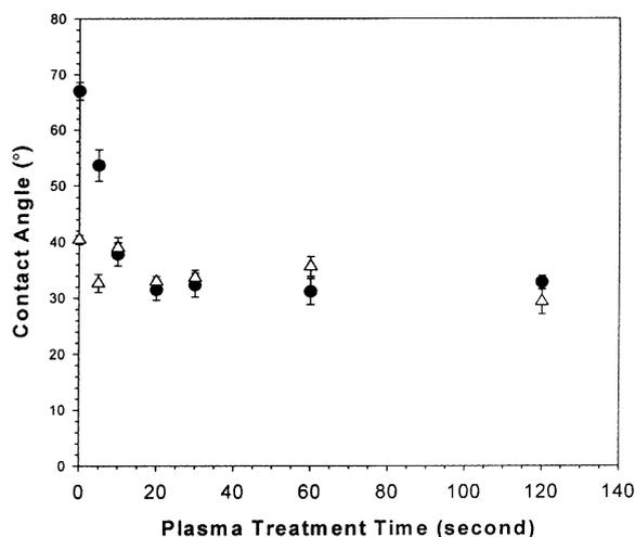
Fig. 3. Contact angle of water (●) and di-iodomethane (△) of oxygen plasma treated polysulfone membrane with the increase of plasma treatment time.
