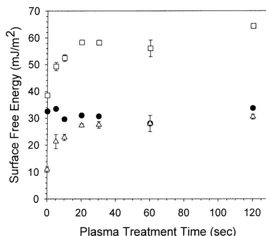
Fig. 4. Surface free energies of oxygen plasma treated polysulfone membrane with the increase of plasma treated time: dispersive component (●), polar component (△), and surface free energies (□).
