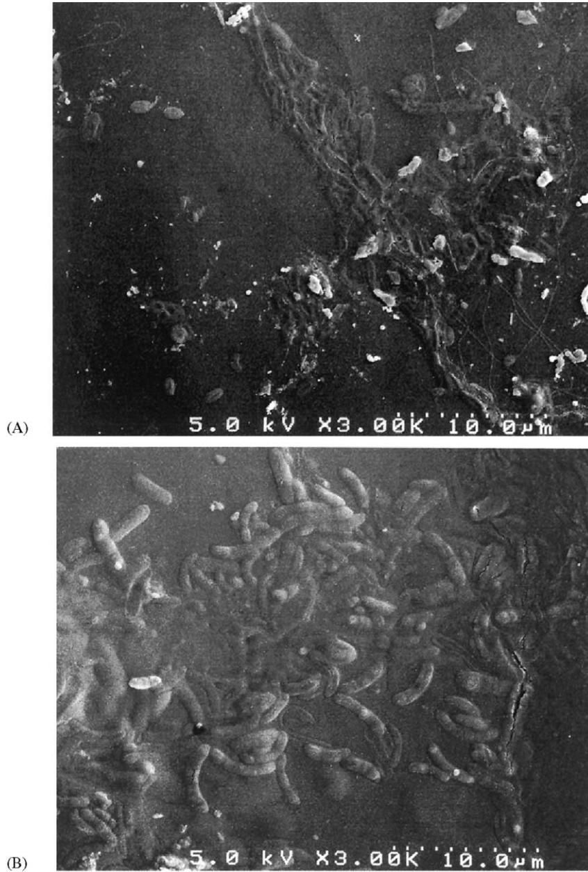
Fig. 7. SEM micrographs of untreated polysulfone membranes at (A) pH 3, (B) pH 8, (C) pH 12 and oxygen plasma treated polysulfone membranes, (D) pH 3, (E) pH 8 and (F) pH 12 after flux test of gelatin solution.
