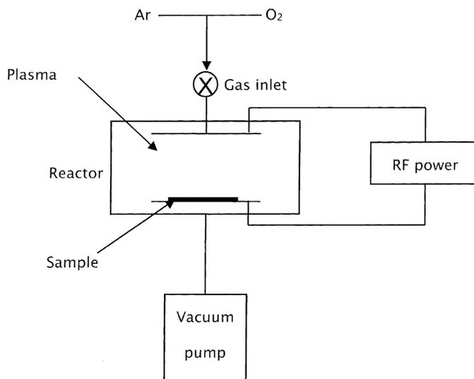
Fig. 2. Schematic diagram of plasma generator.
