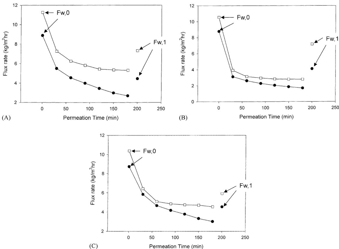
Fig. 6. Flux rate of aqueous gelatin solution at (A) pH 3, (B) pH 8, (C) pH 12: untreated polysulfone membrane (●) and oxygen plasma treated polysulfone membrane (□).
