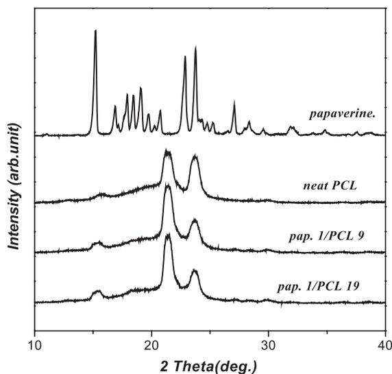
Fig. 3. X-ray diffraction patterns obtained from papaverine, neat PCL microparticles, and PCL microparticles containing papaverine. The neat PCL is a microparticle non-containing drug. The pap.1/PCL 9 and pap.1/PCL 19 are microparticles containing drug in an amount of 4.1 and 2.0 wt.%, respectively.
