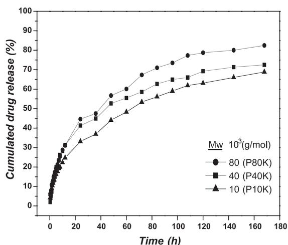
Fig. 6. In vitro drug release profiles from PCL microparticles prepared with a different molecular weight for 1 week.
