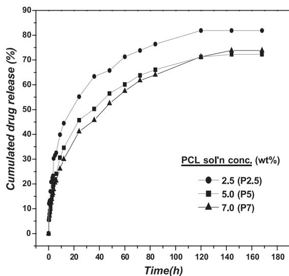
Fig. 5. In vitro drug release profiles from PCL microparticles prepared with a different PCL solution concentration for 1 week.
