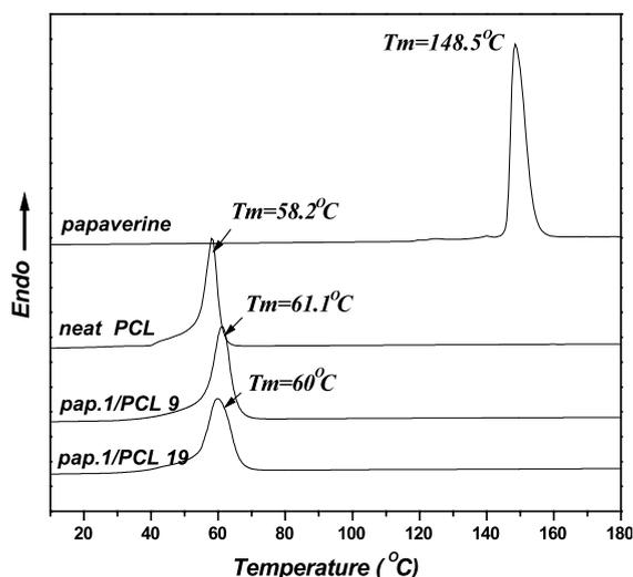
Fig. 2. DSC thermograms obtained from papaverine, neat PCL microparticles, and PCL microparticles containing papaverine. The neat PCL is a microparticle non-containing drug. The pap.1/PCL 9 and pap.1/PCL 19 are microparticles containing drug in an amount of 4.1 and 2.0 wt.%, respectively.
