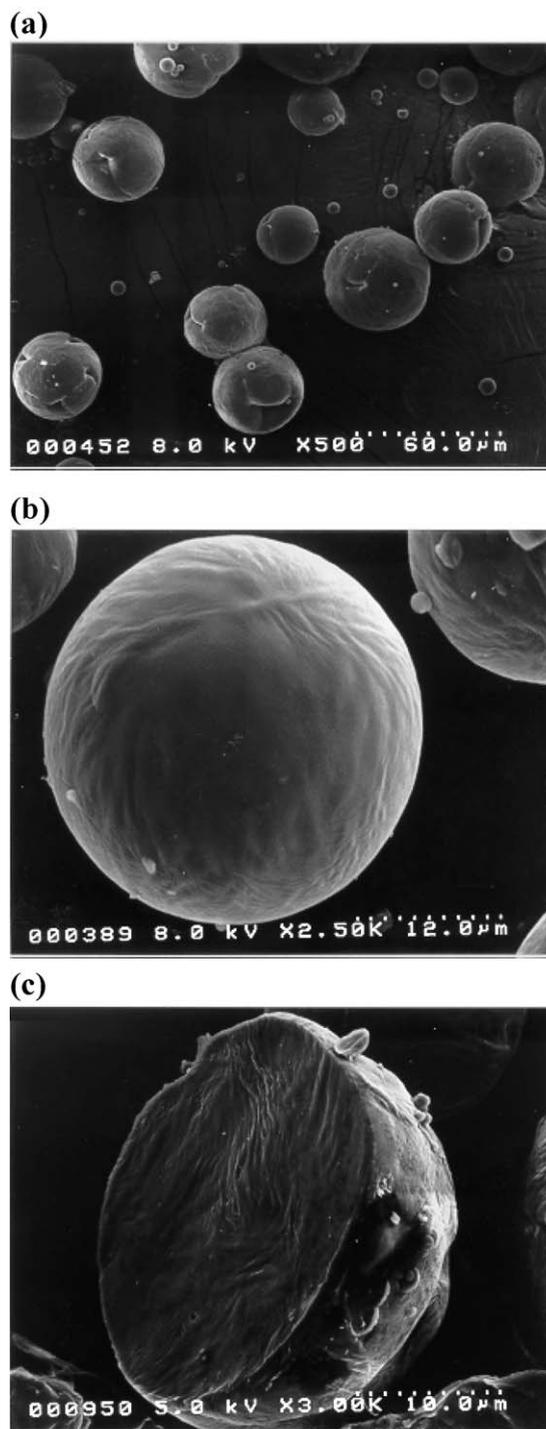
Fig. 1. SEM micrographs of (a), (b) PCL microparticles containing drug prepared by emulsion evaporation technique and (c) cross-section of a PCL microparticles. The microparticles were fixed on support with carbon tape and coated with platinum. In order to observe cross-section of microparticles, the microparticles dispersed in water were frozen and then sectioned using a cryogenic ultramicrotome.
