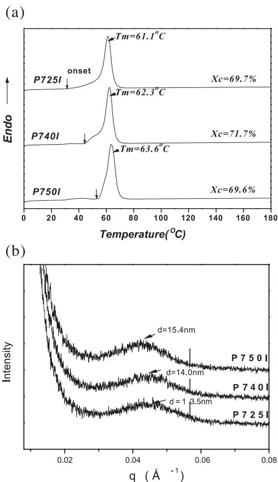
Fig. 4. DSC thermograms (a) and SAXS spectra (b) obtained from PCL microparticles prepared with a different thermal history. The PCL microparticles (P7) were annealed at different temperatures (25, 40, 50 °C) for 3 days.
