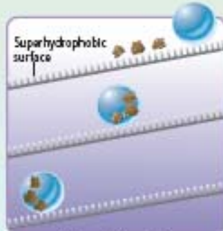
On a superhydrophobic surface, a drop rolls across, picking up dirt and carrying it away. The water and dirt have greater affinity for each other than either does for the surface.
